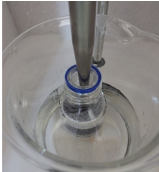
FIGURE 4.1 – Exfoliation du graphite au LPMC.
