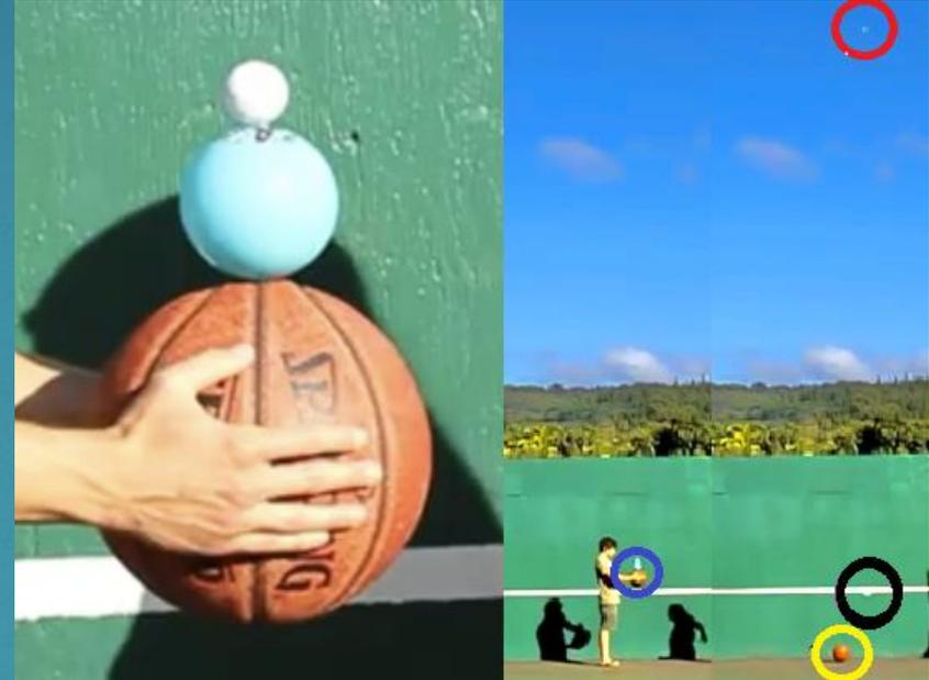
$$\text{Coefficient de restitution : } e = \frac{v_f}{v_i} = \sqrt{\frac{h_f}{h_i}}$$
